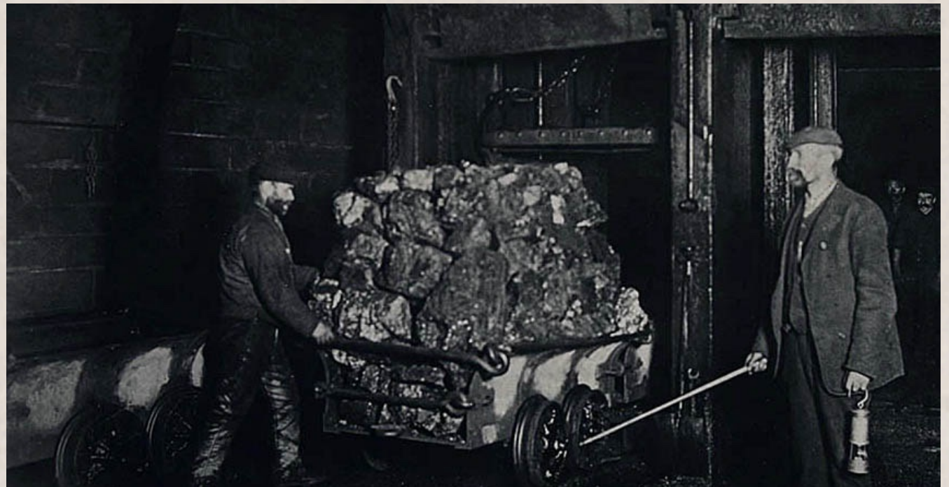
Placing the coal on a tram in the mine
